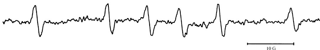
FIGURE 1. ESR spectrum of the reaction mixture (2350 U tyrosinase, 33 mM Met-Gly-NHNHPh*TFA 33 , 90 mM DMPO, O 2 ) after 60 min; a_N = 15.83 G and a_H = 24.55 G, g = 2.0054 .
